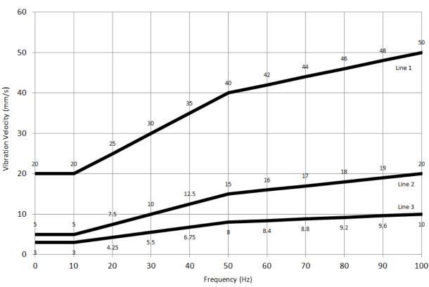
DIN4150 Part 3 "Foundation" Vibration Limits
